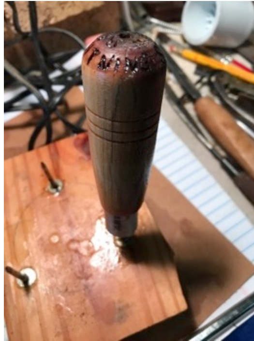
Photo 8: Final result, soaked in polyurethane
