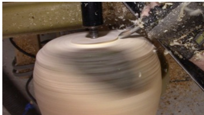
Photo 16: Continuing to trim the blank
