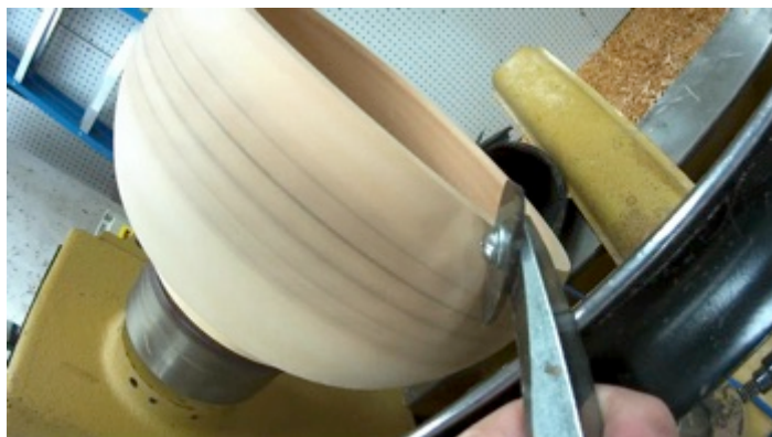
Photo 56: Removing pencil lines by shear scraping
