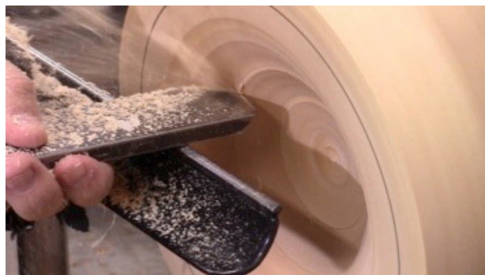
Photo 26: Continuing hollowing with a scraper
