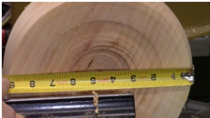
Photo 22: Diameter before drying
