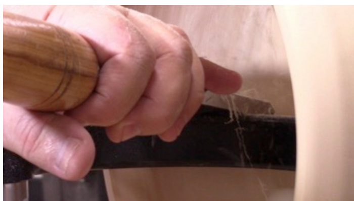
Photo 59: Negative rake scraper on the interior sides
