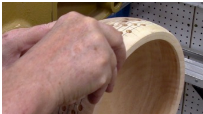
Photo 53: Inserting a peg into the hole, with the narrow end down...
