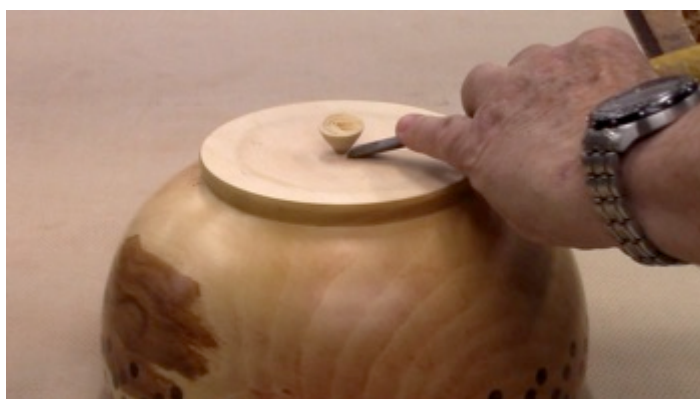
Photo 65: Removing the nub...
