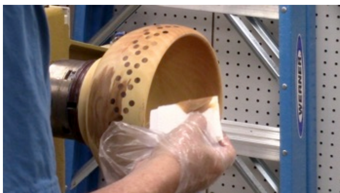
Photo 62: Applying the abrasive grit
