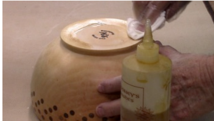
Photo 67: ...and applying some finish to the bottom
