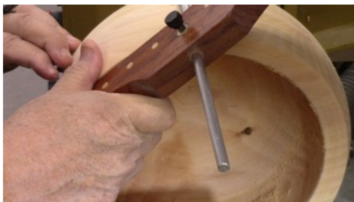
Photo 30: ...then placed over the outside, and the position of the end of the rod is the depth
