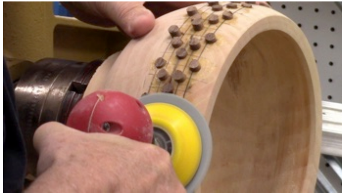
Photo 55: Sanding the pegs flush with the surface
