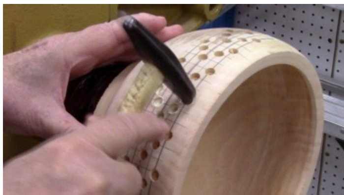
Photo 54: ...and then tapping the peg down as far as it will go
