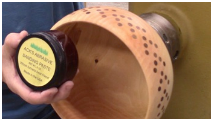
Photo 61: Using Ack's Abrasive Paste after sanding to 240 grit
