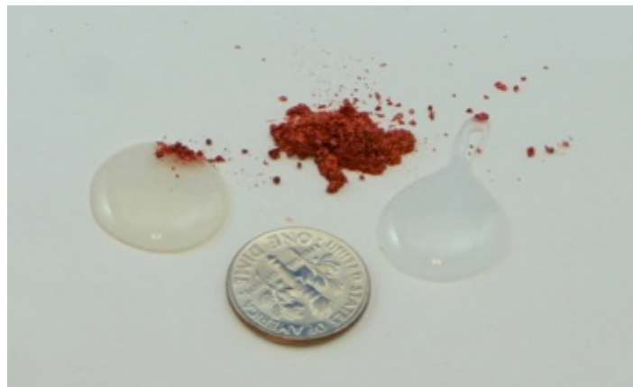
Photo 5: The amount of two-part epoxy and PearlEx™ powder I mix for each application.
