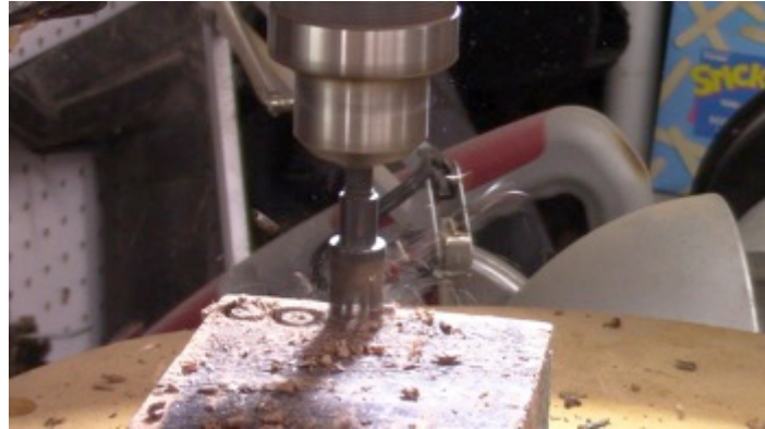
Photo 49: Cutting pegs with a plug-cutter on a drill press
