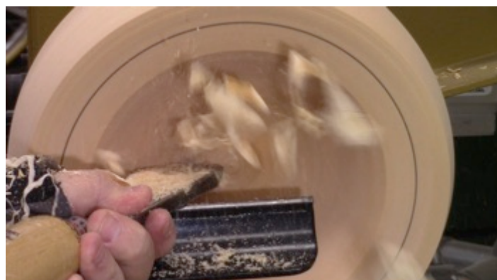
Photo 27: Continuing scraping to deepen the recess
