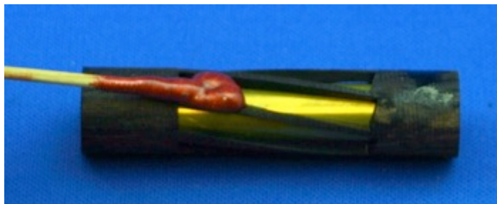
Photo 7: Epoxy and PearlEx™ powder being applied to the voids on a laser inlay leftover.
