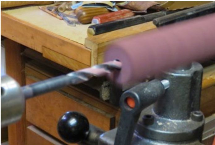
Photo 5: Drilling with aircraft extension bit
