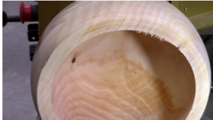
Photo 31: Initial turning is complete
