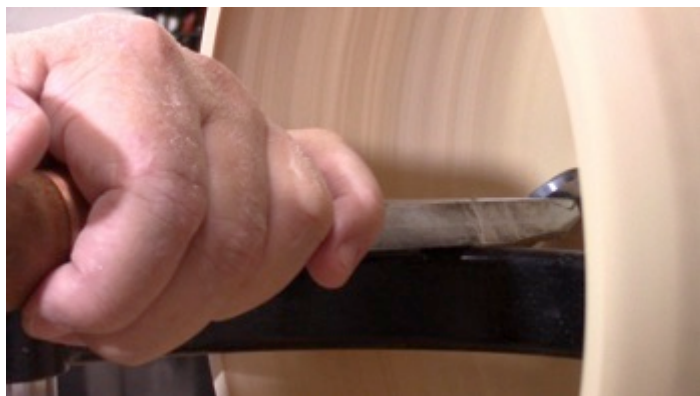
Photo 58: Finishing cuts on the interior of the bowl
