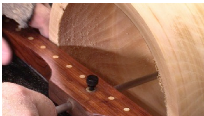
Photo 29: To check the depth, the rod is pushed to the bottom of the bowl...
