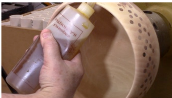
Photo 60: An initial coat of penetrating oil finish
