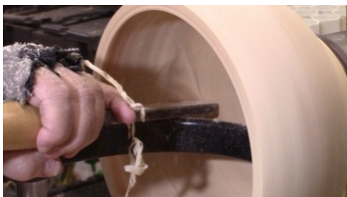
Photo 38: ...and then with a large scraper
