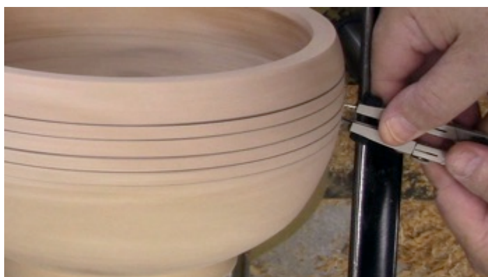
Photo 39: First step in laying out the peg locations
