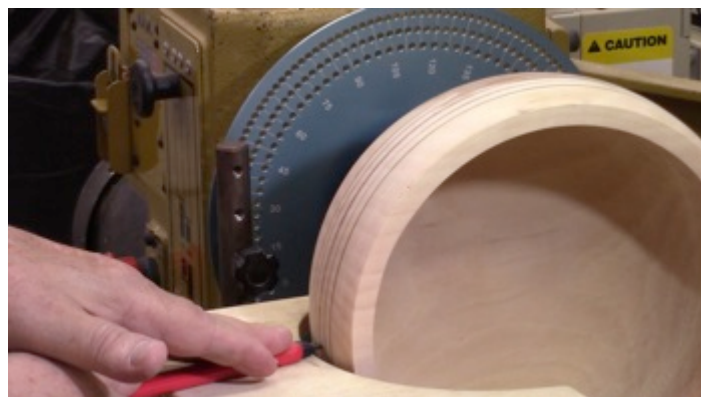
Photo 42: Marking the first indexed line
