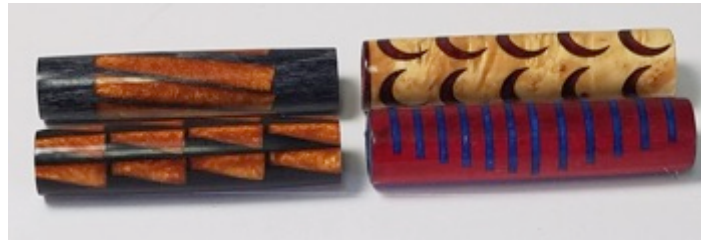
Photo 12: Four other blanks for the sierra pen using laser leftovers and two-part epoxy.
