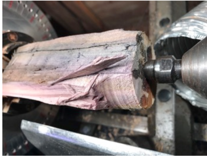
Photo 5: Splitting instead of nice chips...wood tears away
