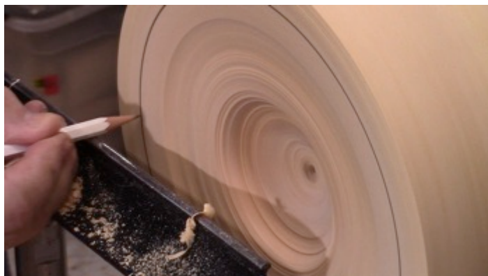
Photo 24: Marking the wall thickness for hollowing
