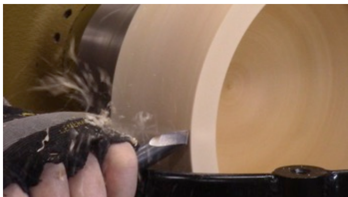
Photo 35: Bringing the bowl blank back into round on the outside...
