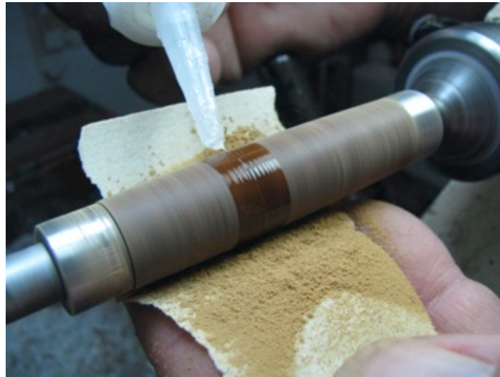
Photo 4: The beginning of the slurry formation.
