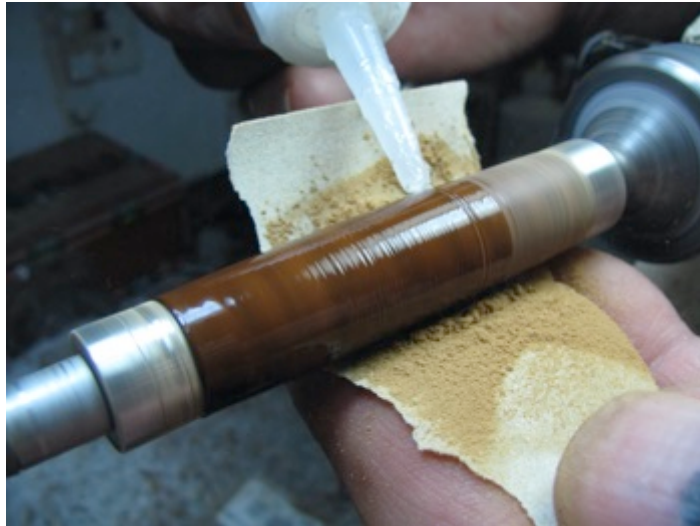
Photo 6: Continue adding CA to mix with the dust to form the slurry.
