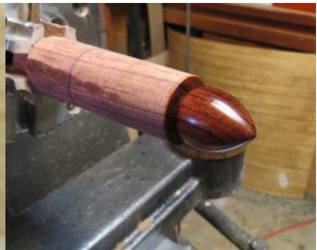
Photo 13: Cap, turned, sanded, finished
