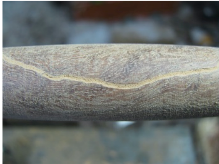
Photo 2: The sanded blank with dust filling the crack.
