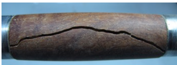
Photo 1: A typical cracked wooden pen barrel
