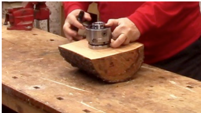
Photo 7: ...and the chuck is expanded into the ring
