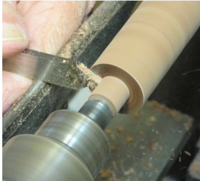
Photo 11: Sizing the tenon for the cap
