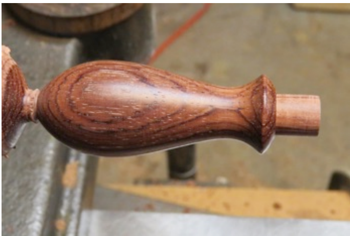
Photo 15: Sanded and ready for finish
