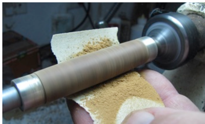
Photo 3: Sanding dust collected on the sandpaper.
