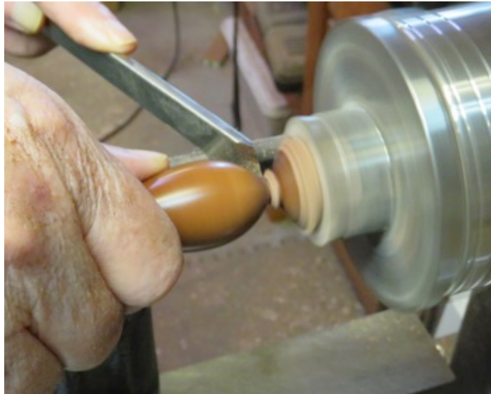
Photo 17: Removing the case from the waste
