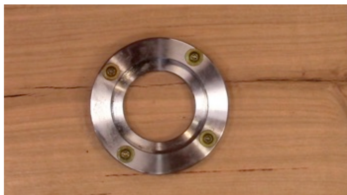
Photo 2: A small (about 3 1/2 inches, 89 mm) faceplate ring
