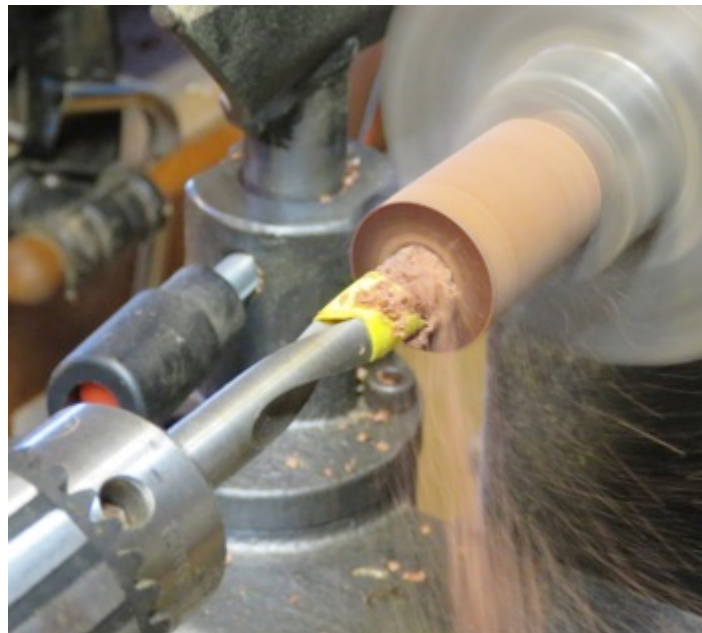
Photo 6: Drilling hole in the cap
